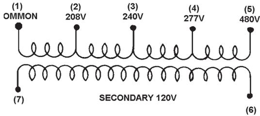
**IMMERSION THERMOSTAT MODEL TRANSFORMER**
